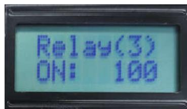
Step 8: Set Relay 3 **OFF** time. Press the set button 1 time (or 9 times if returned to inputs) to advance to Relay (3) OFF:, press the up or down button to change the timing to 105 seconds.
