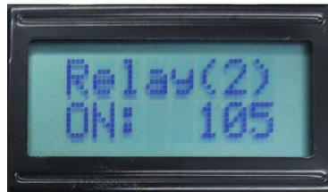
Step 6: Set Relay 2 **OFF** time. Press the set button 1 time (or 7 times if returned to inputs) to advance to Relay (2) OFF:, press the up or down button to change the timing to 120 seconds.
