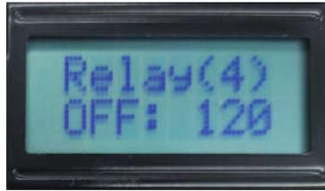
Step 10: Allow display to exit settings and return to Inputs. Do not touch the buttons for 3-5 seconds and confirm the display has returned to normal operation and displays Inputs in the bottom left.
